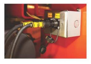
All units utilize Allen-Bradley PLC's and all external control wiring terminated with keyed circular connectors for quick installation.
