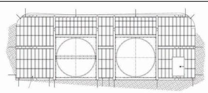
Manual machine doors, powered machine doors, man doors, fan bulkheads and combinations of any of these are possible with the Kennedy system.
